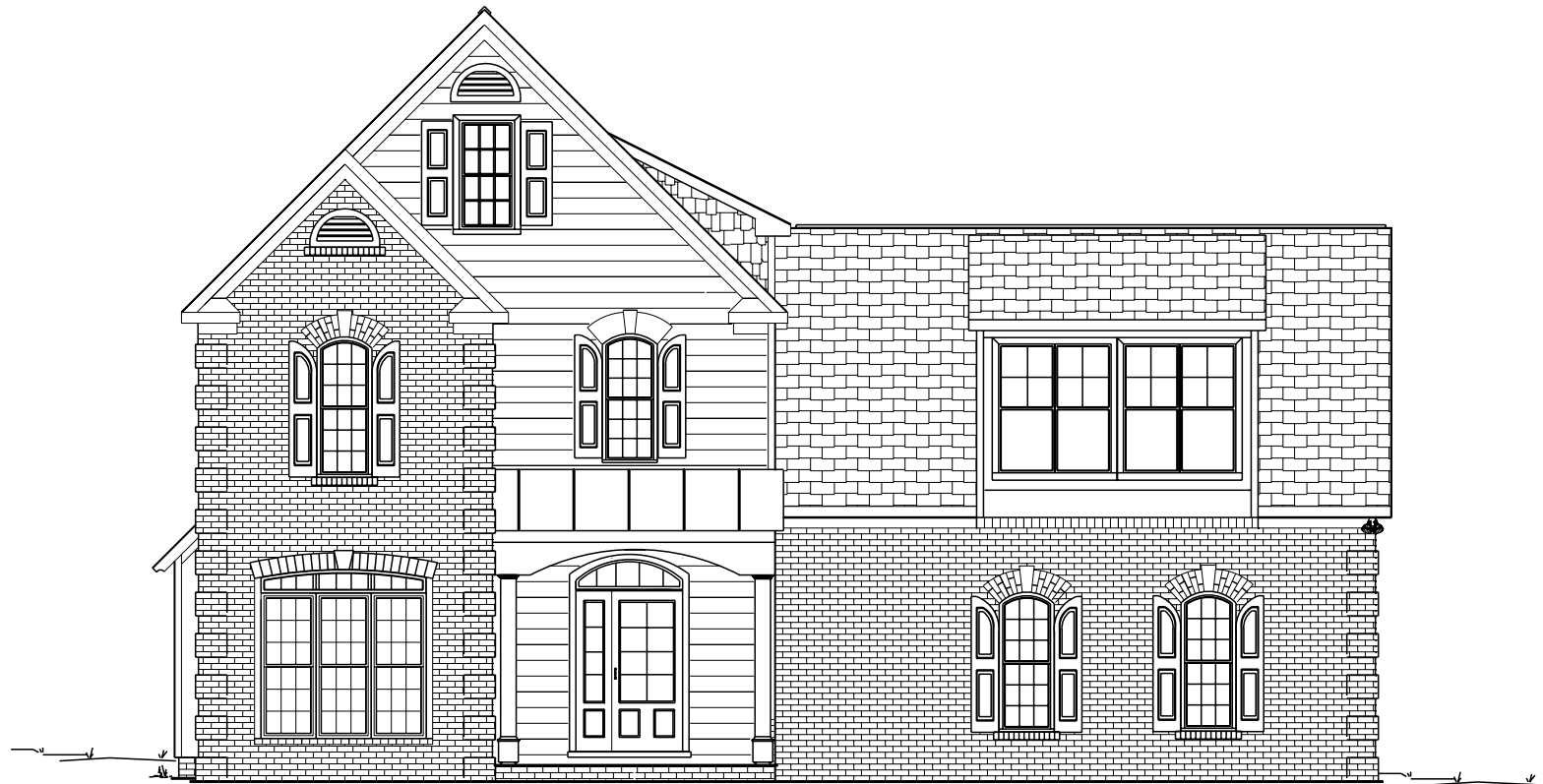
FRONT ELEVATION W/SIDE-LOAD GARAGE
