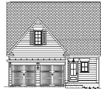
FRONT ELEVATION ( FRONT PORCH EXTENDS 7' BEYOND GARAGE )
